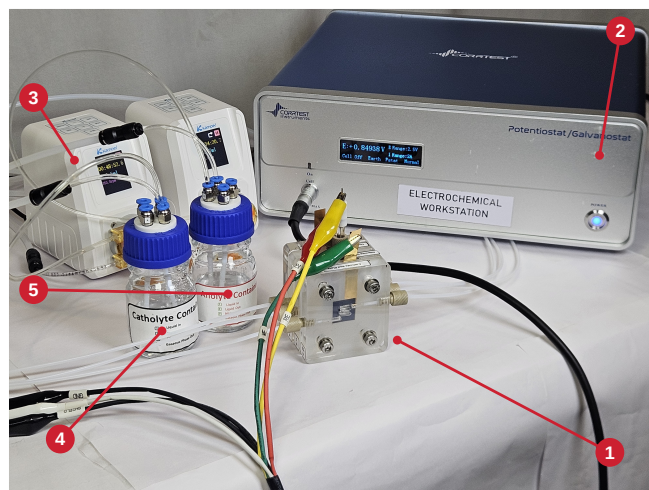
PMMA flow cell connected to dual electrolyte loops and a potentiostat / galvanostat.
